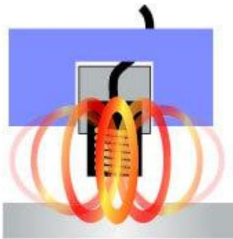
Figure 10 Mounting hardware can interfere with inductive probe magnetic field.
