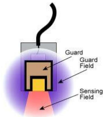
Figure 5 Capacitive probe guarding
