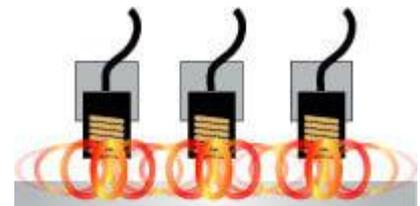
Figure 9 Interference occurs when inductive probes are mounted near each other.
