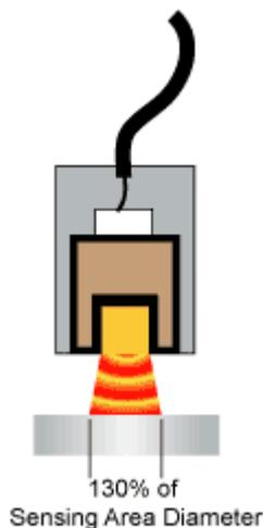
Figure 3 Capacitive probe spot size
