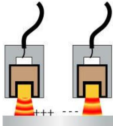
Figure 11 Non-synchronized capacitive sensors will interfere when used on the same target.
