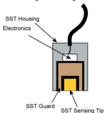
Figure 1 Capacitive Probe Construction
