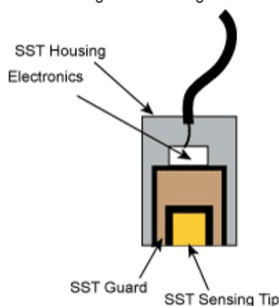
Figure 1 Capacitive Probe Construction
