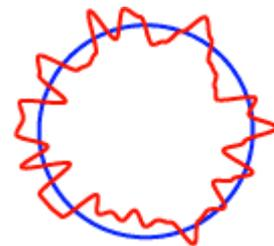
Figure 8 Runout plot showing actual runout in blue, and electrical runout from inductive sensor in red.
