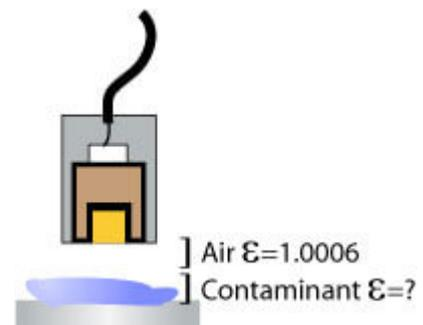
Figure 7 Gap contamination
