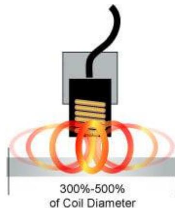
Figure 4 Inductive probe spot size
