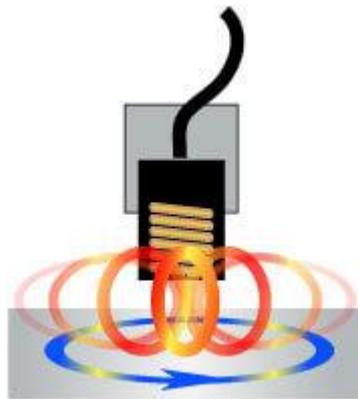
Figure 6 Magnetic field induces eddy current in conductive target
