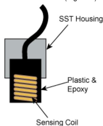
Figure 2 Inductive Probe Construction
