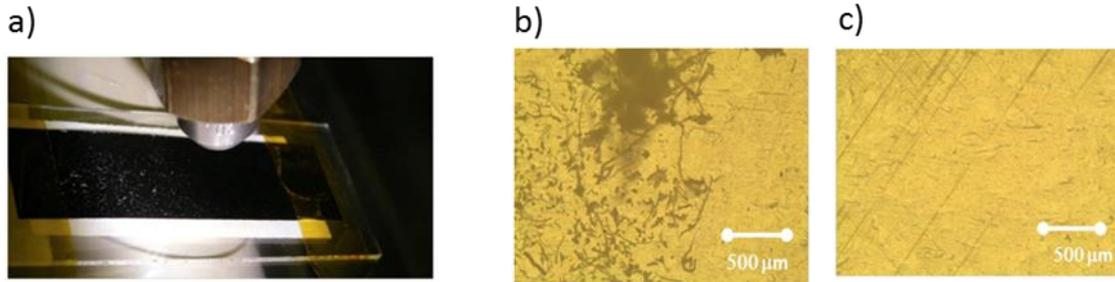
Figure 4.4 a) N<sub>2</sub> gas nozzle on R2R line at TNO b) coated paper pre-cleaning c) post-cleaning
