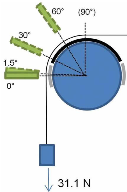
Detailed investigation of the form of the foil as it moves over the air turn has allowed for simulation models to be developed. From these models optimum configuration of the air bearings has been identified for in-line use, including air turns with dual zones (Figure 11).
