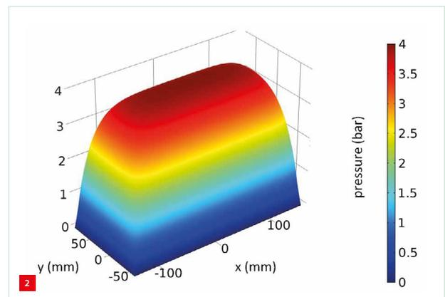
constantly escaping from the bearing gap. The restriction maintains the pressure under the bearing and supports the working load. It is used to optimise the bearing with respect to lift, load, and stiffness for particular applications.
