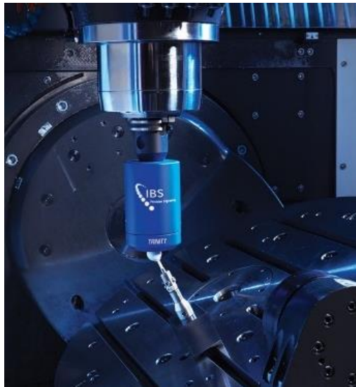
Figure 1. Photo of measurement setup of Rotary Inspector, combining a 3D wireless probe with a precision master ball on a 5-axis machine tool.
