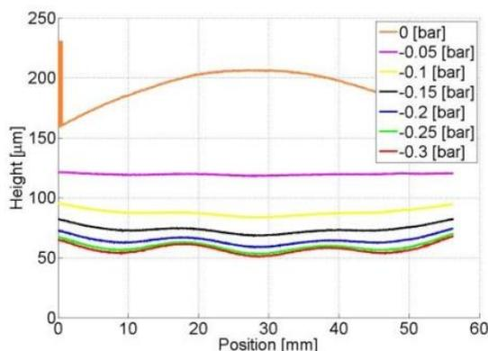
Figure 3. Web flatness over the width of the air table, the length of the web using 2 bar air pressure, 0 to -0.3bar vacuum.
