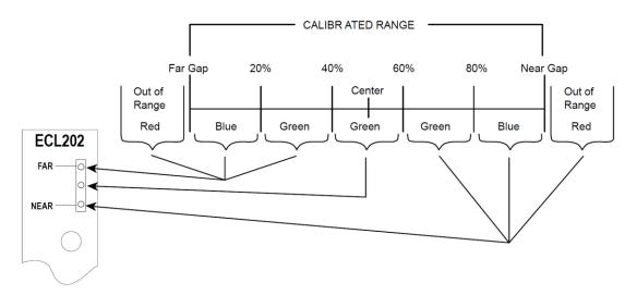
The LED Range Indicator is independent of the output voltage and not affected by the Offset button. Shifting the output voltage by using the Offset button may allow an apparently valid output voltage to exist while the probe is out of range. When the Near or Far LED is red, the probe is out of range and the output voltage is not a reliable indication of the target position.
