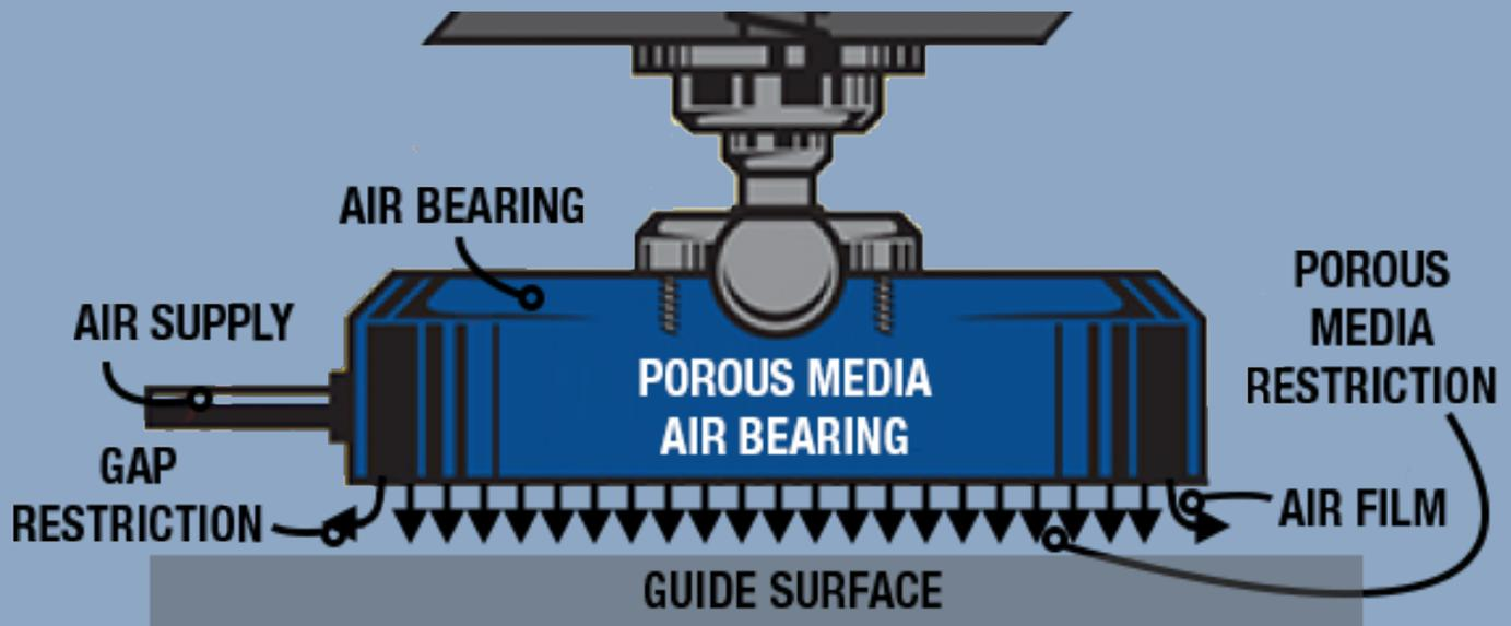
Air Bearings can be used for various **precision motion and positioning applications** in vehicle testing:
