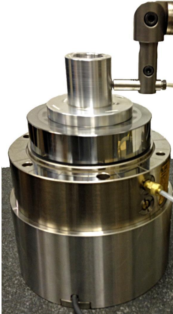
Figure 5 Measurement of the out-of-roundness of an aluminium target using a Lion Precision C1-C capacitive sensor.
