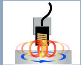
Magnetic field induces eddy current (blue) in conductive target
