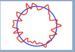
Actual runout (blue), and electrical runout from ind. sensor (red).
