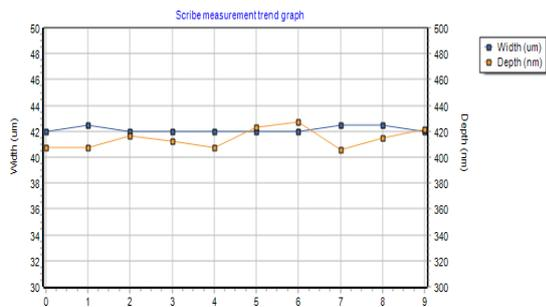
Figure 11 Trend graph of laser scribe and width taken in-line.
