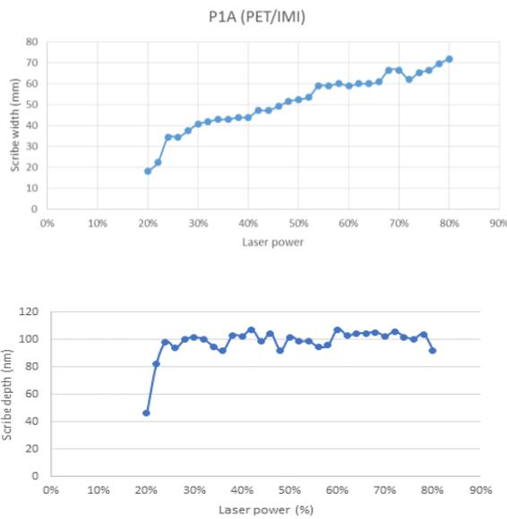
Figure 9 Measured P1A scribe width (upper graph) and depth (lower graph) as a function of laser power.
