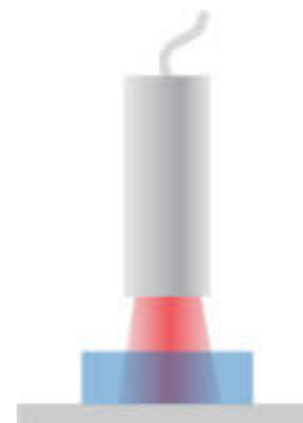
Figure 7 Non-conductors can be measured by passing the electric field through them to a stationary conductive target behind.
