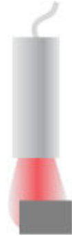
Figure 8 An undersized target causes the sensing field to extend to the sides of the target, introducing error
