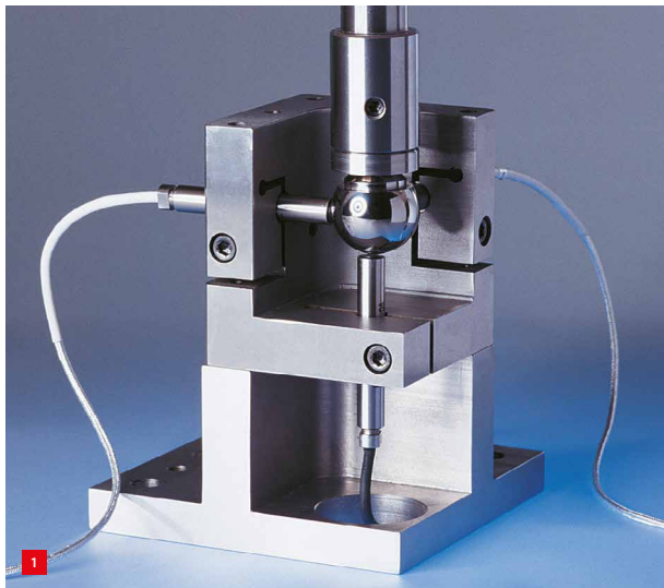
Set-up of a classic thermal distortion test using three capacitance sensors.
