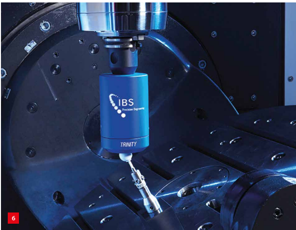
Rotary Inspector set-up: 3D probe in spindle, masterball on the table.
