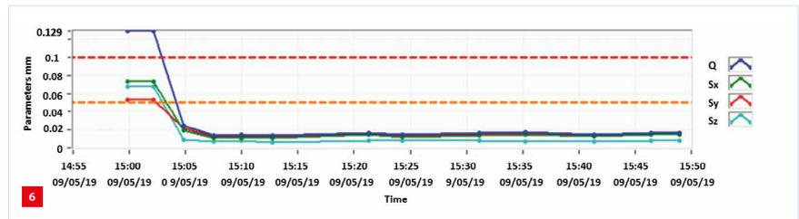
Typical Rotary Inspector output, showing the evolution of the Q value, i.e. the maximum geometrical error, and the underlying maximum individual axis errors (Sx, Sy and Sz). The sharp decline in all values reflects the error compensation taking effect.
