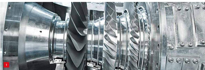
Turbine manufacturing at MTU is a high-complexity, high-precision process requiring true 6-axis grinding.
