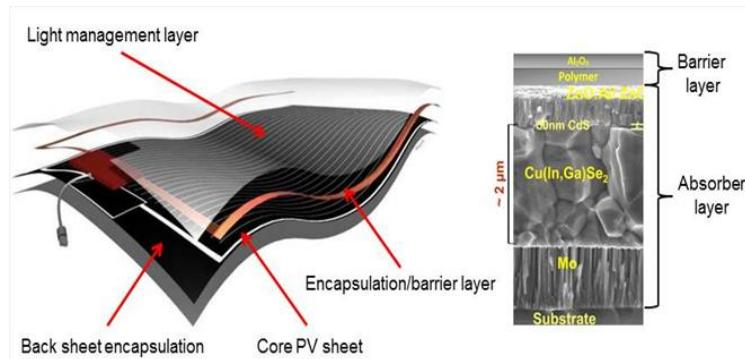
Figure 3.2 Function layers in flexible PV substrates (courtesy Flisom)
