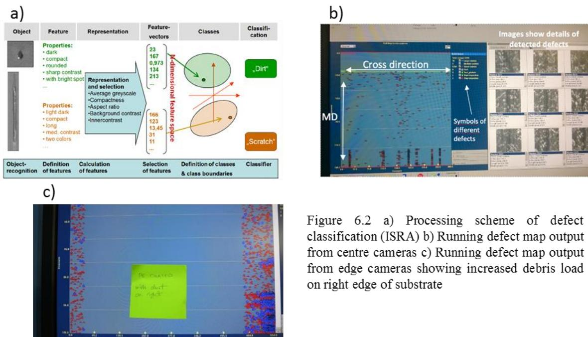
Figure 6.2 a) Processing scheme of defect classification (ISRA) b) Running defect map output from centre cameras c) Running defect map output from edge cameras showing increased debris load on right edge of substrate
