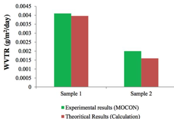
Figure 3.4 Comparison between the theoretical at (3μm lateral cut-off) and experimental WVTR results for two tested samples
