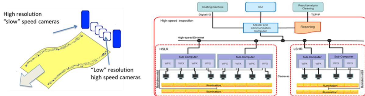
Figure 5.4 a) Schematic setup of the hybrid system at TUT b) Computer hierarchy adopted to deal with high data rates
