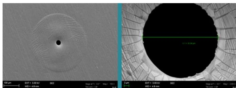
Figure 3.5 Laser drilled pin hole defects in Paper/LDPE/ALD substrate
