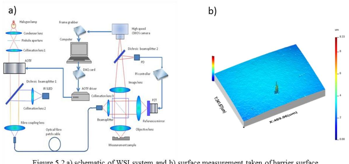
Figure 5.2 a) schematic of WSI system and b) surface measurement taken of barrier surface
