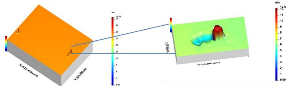
Figure 6.4 Measured surface containing significant defect exploded defect view. In situ coated film measurement, inset image 50 x 25μm
