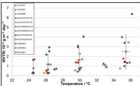
**Due to the lower detection limit of the AQUATRAN 1 system the NPL cavity ring-down spectroscopy (CRDS) method, (to be reported later) was used to measure accurate WVTR values for single ALD barrier layers on planarised PEN. The lower detection limit for CRDS is  $3 \times 10^{-5}$  g/m<sup>2</sup>/day.**
