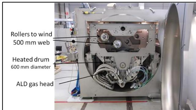
Figure 2.3 – R2R ALD tool (inside vacuum chamber)
