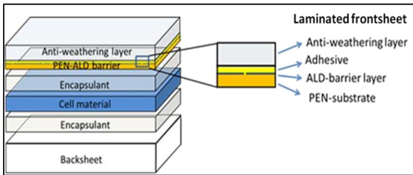
Figure 2.2 – Cross section of the Isovoltaic frontsheet including produced ALD barrier layer
