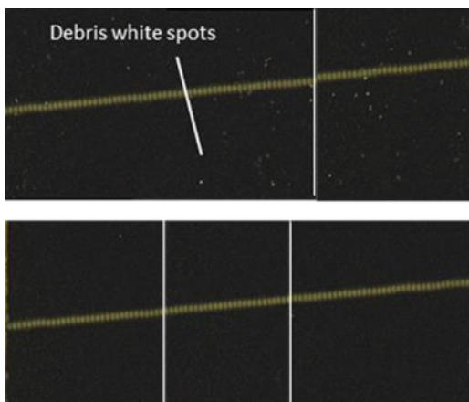
Figure 4.3 Optical microscope images of scribed Mo film with redeposited Mo particles before and after ( $1\text{ l min}^{-1}$  N<sub>2</sub> gas jet cleaning at a nozzle – substrate angle of 45°, a distance of 2 cm and a web speed 2 m/min).
