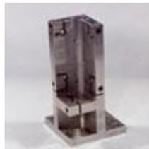
2X, 2Y, and Z measurements for tilt and error motion with 5-channel systems.
