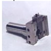
Fits in turning centre tool holder and holds a standard three probe nest.
