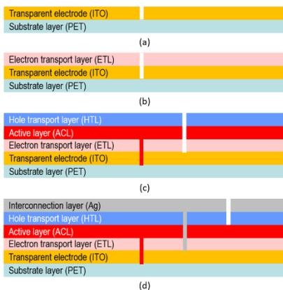
Figure 7 Schematic representation of the organic electronics stack, with (a) the P1A type, (b) the P1B type, (c) the P2 type, and (d) the P3 type laser scribes
