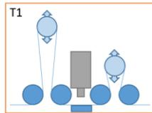
Figure 2 Schematic of dancer. Dark blue -standard rollers, light blue- cylindrical porous media air bearings (airturns).
