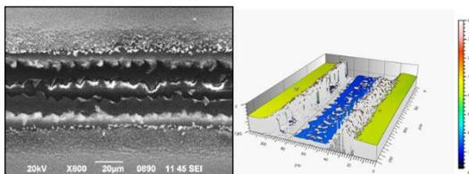
Figure 8 Comparison between SEM image (left) and ARINNA interferometer measurement (right) for P3 scribe.
