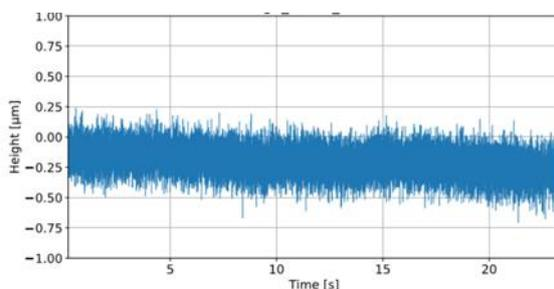
Figure 6 z-stability of web during dancing and stabilisation with air table.
