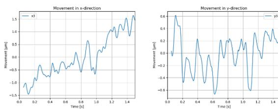
Figure 5 Left: x-position of laser scribe on web during dancing (std. dev.  $0.8\mu\text{m}$ ). Right: y-position (std. dev. of  $0.3\mu\text{m}$ ).
