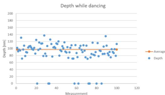
Figure 12 100 scribe measurements measured in-line at 1m/min.
