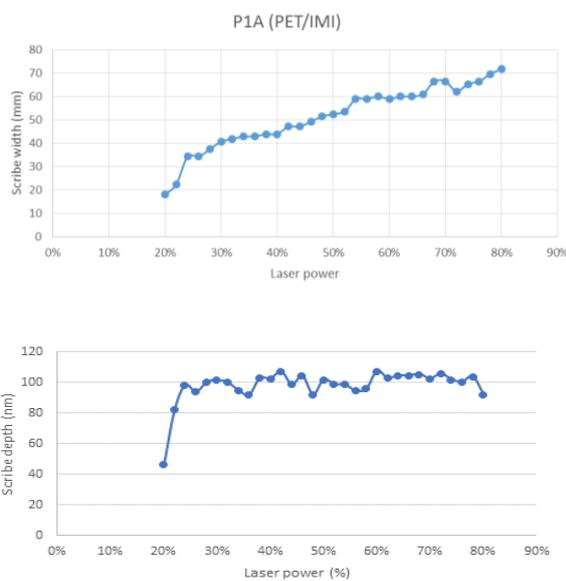
Figure 9 Measured P1A scribe width (upper graph) and depth (lower graph) as a function of laser power.
