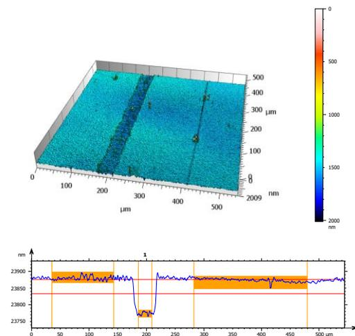
Figure 10 P1A scribe in PET/ITO on foil moving at 1m/min
