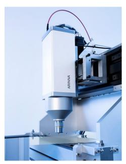
Figure 1 ARINNA interferometer
