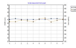
Figure 11 Trend graph of laser scribe and width taken inline.
