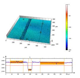
In Figure 10 measurement of a P1A scribe on PET/ITO is shown, measured in-line with a foil speed of 1m/min. Cross-section shows a scribe depth of 100nm in line with the expected ITO layer thickness.
