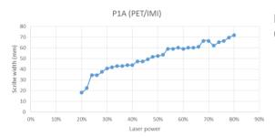
Figure 9 Measured P1A scribe width (upper graph) and depth (lower graph) as a function of laser power.
