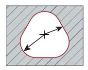
SCA/SEA: Radial Synchronous Error Motion
