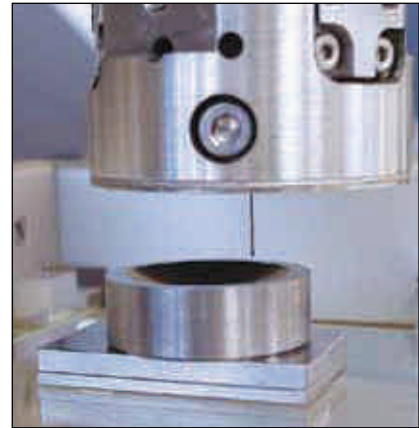
Figure 2.2: Measurement of aspherical mould insert
