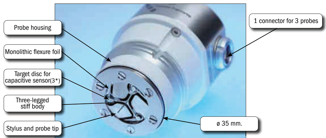
Figure 1.2: Design of the Triskelion ultra-precision touch probe.
