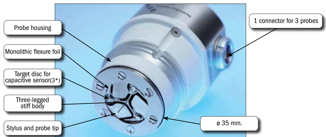
Figure 1.2: Design of the Triskelion ultra-precision touch probe.
